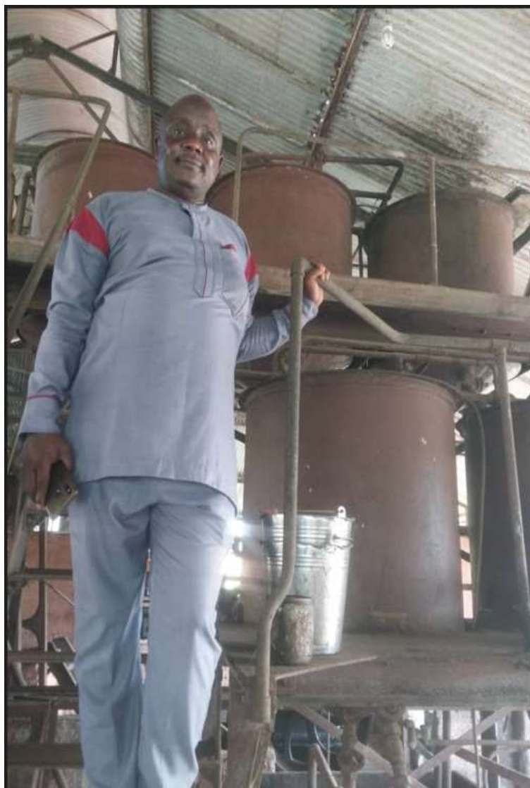
An Artisanal Fabricator with a Locally Fabricated Oil palm fruits Boiler Tank by Dantale at Anyigba Dekina LGA, Kogi State
